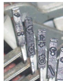
Fig. 2. An Olympia portable typewriter (ca. 1968) altered to type Old English.
