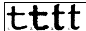
Fig. 7. 1. Typed on a Selectric; 2. printed on a dot-matrix printer; 3. printed on an HP LaserJet II; 4. printed on a LaserJet 1200.
